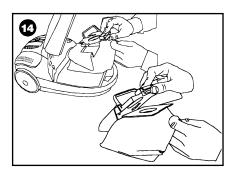
Your appliance is equipped with a dust bag. If you notice that the vacuum cleaner seems to be less efficient than usual, check the dust indicator by selecting the maximum power and lifting the cleaner tool off the floor. If the indicator turns red, change the bag.
